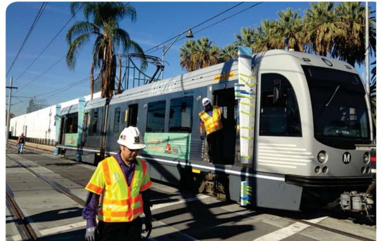
In December 2014, the first two-car train was brought to the Foothill Gold Line to support testing of the new light rail line. A $4 million AnsaldoBreda P2550 weighing over 100,000 pounds was outfitted with specialized gear to test clearances, wheel/rail interface, rail switches, and the Overhead Catenary System.
