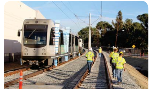
Clearance testing is performed at a walking pace to ensure there are no obstructions in the LRV's path. Note the foam boards placed on the LRV to simulate the worst case scenarios of cab movement.
