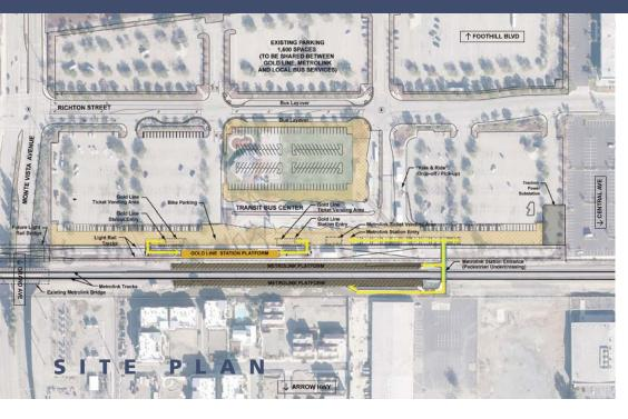
The Montclair station will be located at the Montclair TransCenter, just east of Monte Vista Avenue and north of Arrow Highway. The Gold Line station will be a center platform station, with light rail tracks on either side (one for westbound and one for eastbound trains) and will be located to the north of the existing Metrolink platforms. A connection will be built between the Gold Line and Metrolink platforms via the existing pedestrian tunnel to facilitate pedestrian movement between systems.
